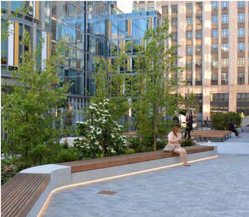
The design proposes one light multi-fixture pole in the northeastern corner. Floodlights would be attached to the shade structure poles, and would be separately controlled for everyday lighting and stage lighting during events. Strip lighting would accent seating elements and the shade structure beams (see renderings).
